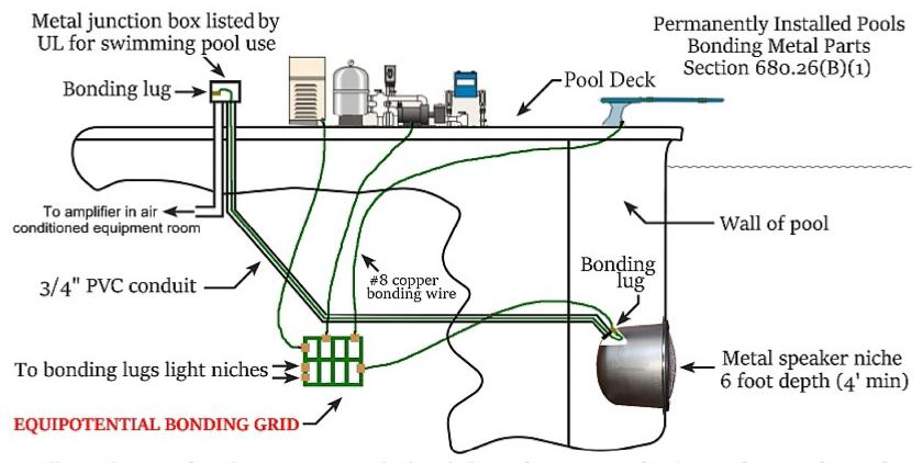
All metal parts of pool structure must be bonded together. Nonconductive steel cannot be used because it does not eliminate voltage gradients.
