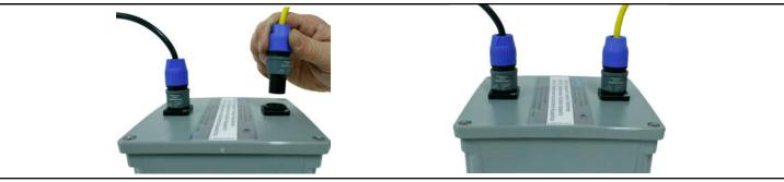
12. Plug the Diluvio Speaker cable connector into the transformer output. Make sure to turn the connector until it locks in place.
