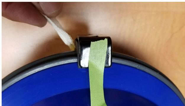
6. Position C3 cage face down on table *with integral mounting bracket facing down*. (If this is up, speaker assm will be blocked from sliding into receiver rails.)
