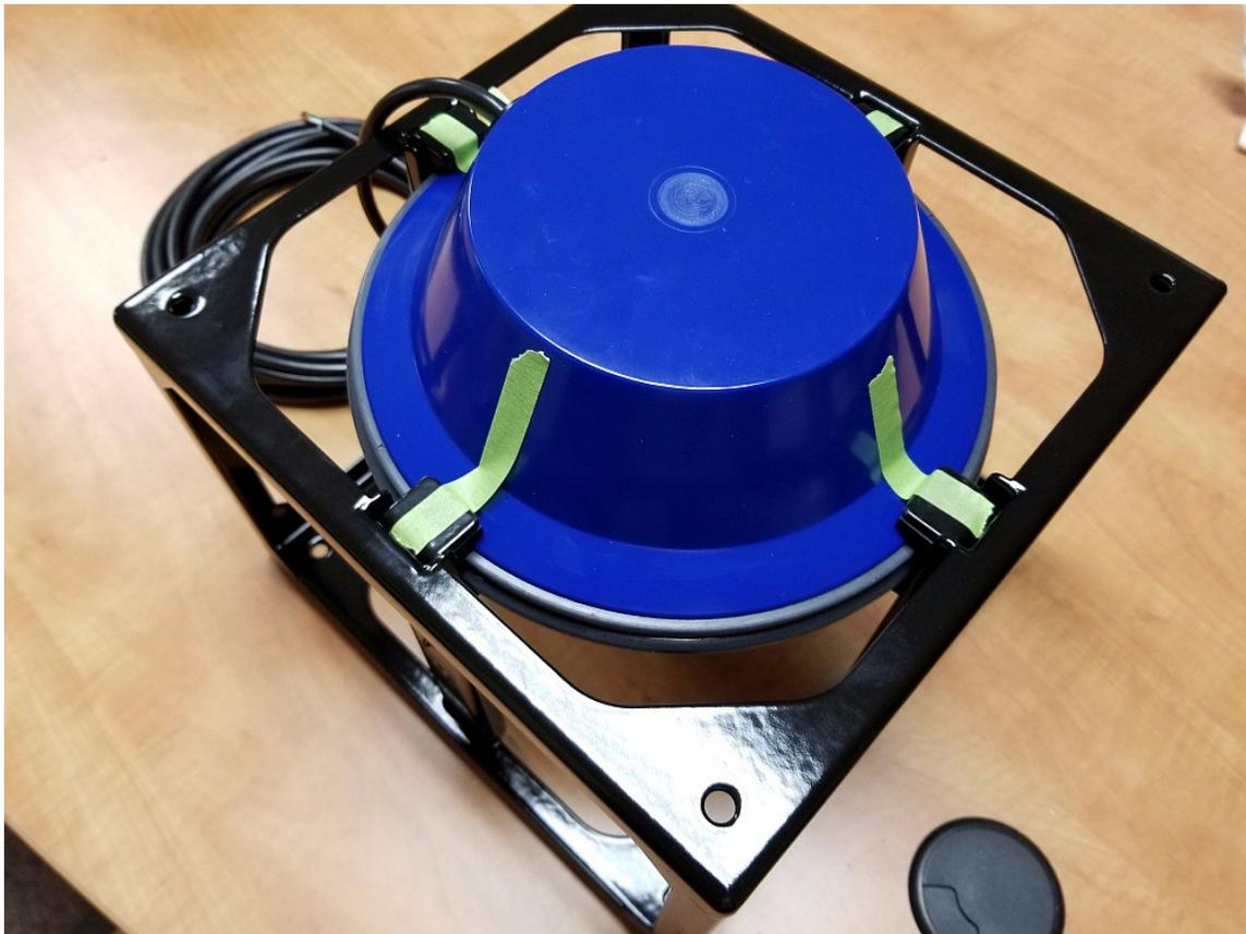
9. Install seven 10-32 x ¼ inch screws, leaving one out on the top of the cage.
