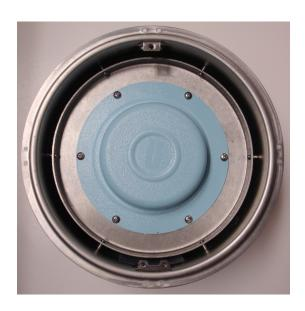
Step 3: Pull UW30 speaker cable thru conduit to J-box. Seal conduit opening in niche per code as required. Insert speaker and install six 10-32 x ½ machine screws.
